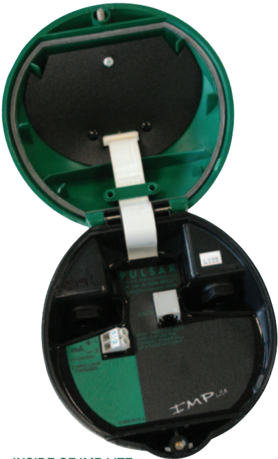
INSIDE OF IMP LITE SHOWING RJ11 PORT
