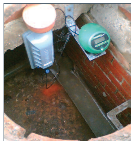
IMP MONITORING IN A CSO CHAMBER
