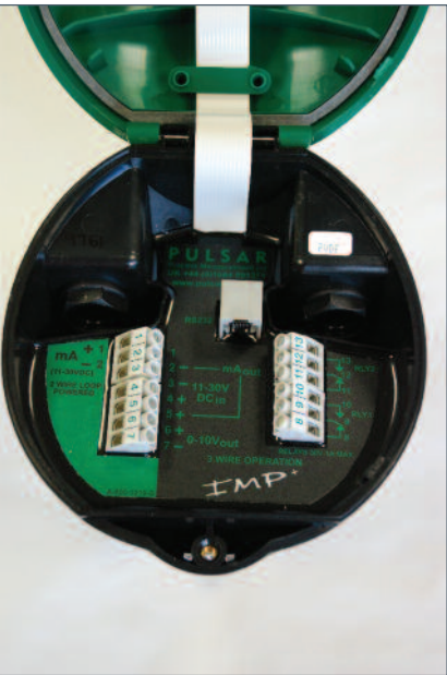
INSIDE OF STANDARD 2/3 WIRE IMP
