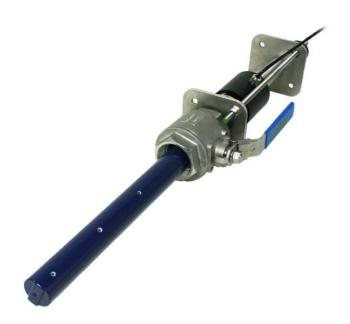
The AVI-Mag<sup>TM</sup> is a hot tap full profile electromagnetic insertion flow meter. Multiple electrodes placed across the entire sensor body at **equal area**, measure and report the average flow rate over the full diameter of pipe. The specific design of the multi-electrode sensor compensates for variable flow profiles, including swirl and turbulent condition.
